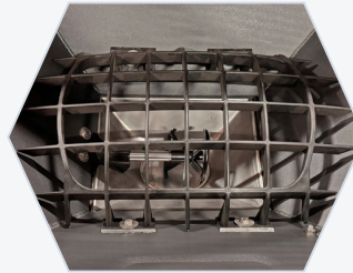
Inox mixer, inox fertilizer mixing chamber and flow router
